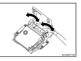
When connecting the hybrid vehicle control ECU harness connector, fasten it securely with a lever as far as it will go as
