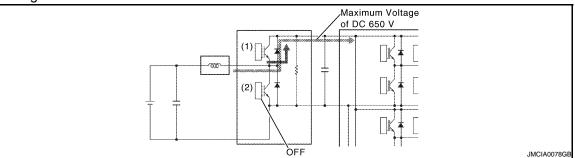
Induced by the counter electromotive force that is created, the electrical power (maximum voltage of DC 650 V) that is charging the reactor flows into the inverter.
