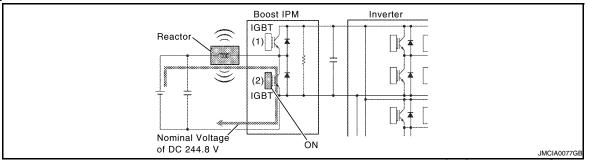
• In the next stage, when the voltage in the reactor rises to maximum voltage of DC 650 V, the IGBT (2) turns OFF, causing a counter electromotive force to be created.
